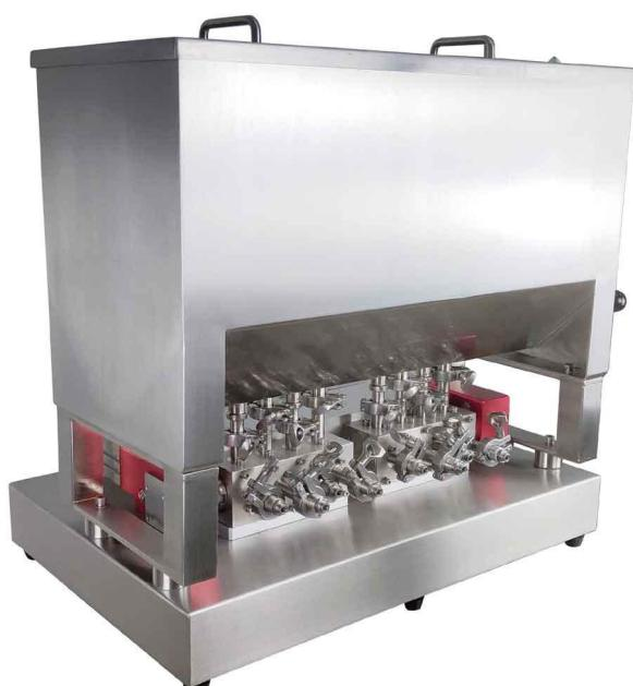
**HBD-10R-6** is a filling equipment that integrates Q-R series ceramic pumps and large-capacity hoppers. It can be equipped with a control system according to requirements, and is widely used in automatic packaging equipment for various cream materials.
